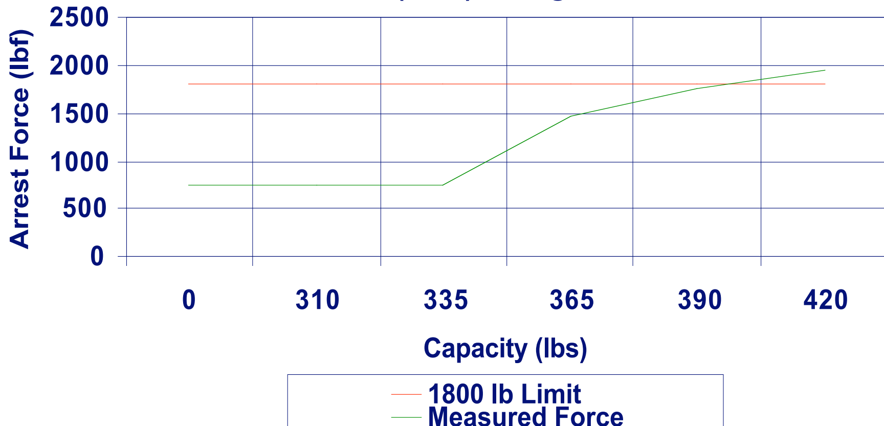
Arrest Force vs Increasing Capacity 900 lb (4KN) Design
